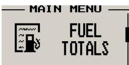
These are 2 independent accumulators for fuel tank 1 and fuel tank 2 that totalize the amount of fuel burn since the last time the accumulators were reset to zero.
