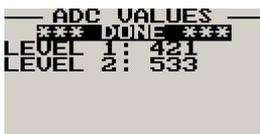
This menu displays the ADC values that have been read from the two fuel level senders.
