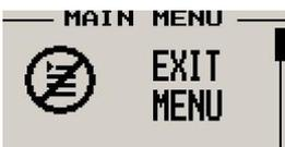
Pressing the rotary control on this menu item will cause the FF-3 to exit the menu system. All changes made during navigation of the menu system will be saved in non-volatile memory on exiting the menu system. If you remove power before exiting the menu the instrument will not save any changes.
