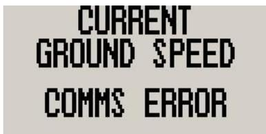
Pressing the F1 key during the main display will show the current airspeed (using the ASX-1 indicator) or ground speed (using a NMEA enabled GPS receiver). This value is used for fuel range calculations.
