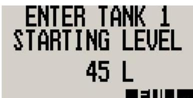
Press the F2 key during the main display screen to manually enter your current fuel level after fueling or defueling your aircraft. This function is only available if you have a mode selected where fuel level is calculated from fuel flow. Press the F2 key again as a "quick fill button" to the full level.
