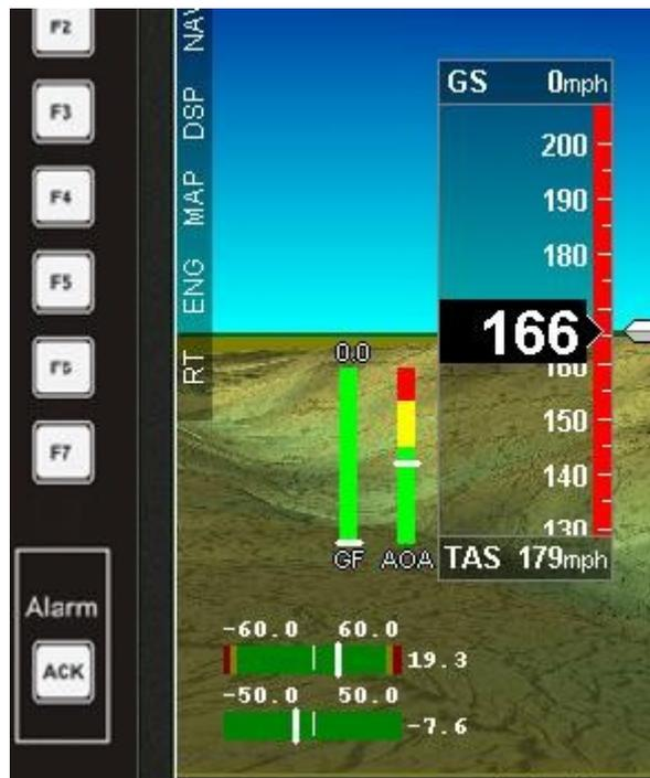
We assume you are familiar with the Screen designer. Here we placed two horizontal “bug bargraphs” on a screen and attached these to the two sensors. We used the built in numeric readouts. We could also have used “special text” items to display the numeric readouts in a different position if required.
