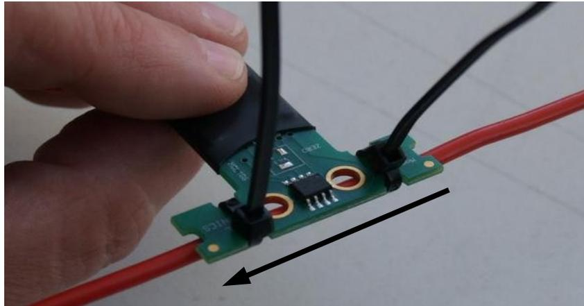
This image shows the direction of current required for a positive (+) reading. Please note that this image shows the wire BELOW the sensor. If the wire were ABOVE the sensor the reading would be negative (-) as the sensor chip would see the magnetic field from the reversed direction.
