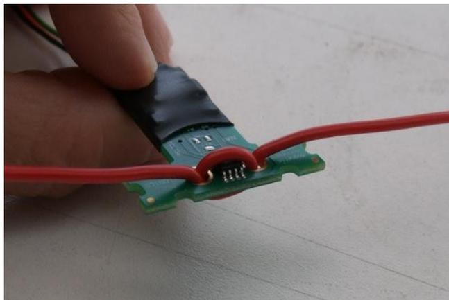
This variation uses 1.5 windings of AWG 18 (1.0mm) wire. This results in a measurement range of +/-12A with good resistance to external magnetic interference.
