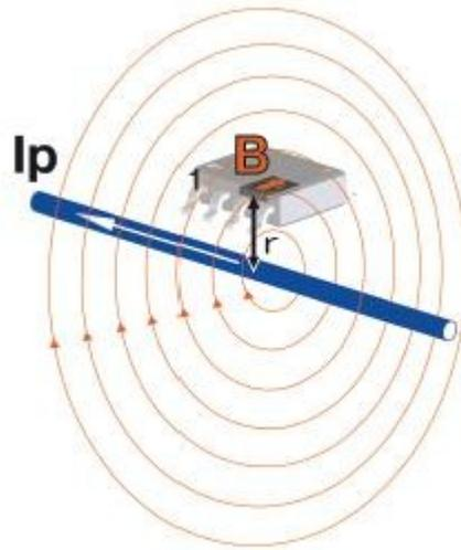
The magnetic sensor chip contains a hall effect sensor array placed on a magnetic flux concentrator. Tiny changes in the magnetically influenced properties of the hall effect sensors are amplified and processed and made available to external circuits.
