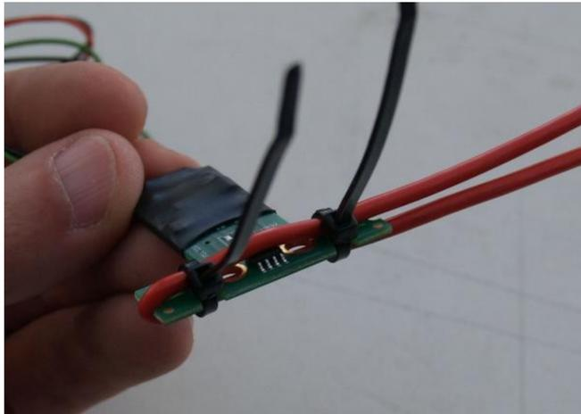
This variation folds a AWG14 (1.6mm) wire over the sensor (effectively one winding).
