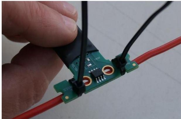
This configuration attaches the sensor onto a AWG 14 (1.6mm) wire.
