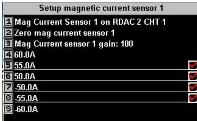
We now need to set the “zero current” measurement point for our magnetic current sensor. Ensure that either there is not current through the attached conductor or remove the sensor from the conductor and then select “Zero mag current sensor 1”. If you have a readout for the current on the screen at this time, you should now read 0.0A. Move the sensor around slightly to confirm that there are no stray interfering magnetic fields affecting the reading.
