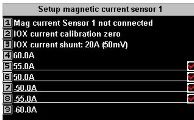
If no magnetic sensor 1 is selected, the G2 defaults to the IOX current shunt for current 1. The first thing we do is assign CHT1 on RDAC2 as source for current sensor 1.
