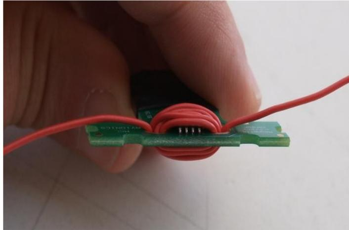
This configuration wraps 7.5 turns of AWG 25 (0.5mm) wire around the sensor. This results in a low range of about +/- 4A that is very resistant to stray magnetic interferences.
