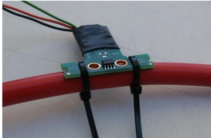
This configuration attaches the sensor to a high current cable such as used for an engine starter motor.
