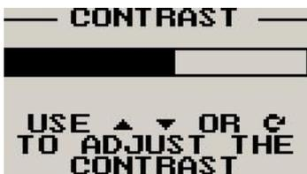
Use the up and down keys or the rotary control to adjust the display contrast.
