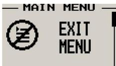
Pressing the rotary control on this menu item will cause the TP-1 to exit the menu system. All changes made during navigation of the menu system will be saved in non-volatile memory on exiting the menu system. If you remove power before exiting the menu the instrument will not save any changes.
