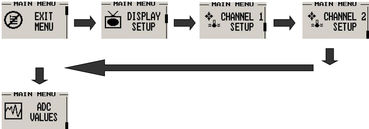
**Note:** “ADC Values” menu item is only visible when switching the unit on and pressing the rotary control. The text “CALIBRATE” will appear on the intro screen when entering this mode.
