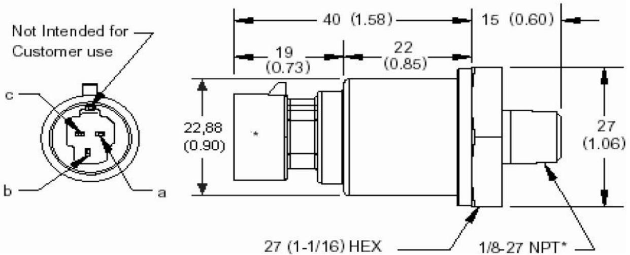
The sensor cable is approximately 3m long and has 3 leads. The black lead is not to be connected and has no function. The Red lead from the sensor has to be connected to the positive bus via a fuse or circuit breaker . The white lead (Output signal) has to be connected directly to the TP-1 Yellow wire (Pin 8).
