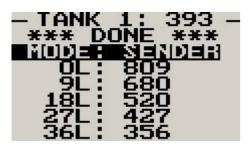
The fuel level sender needs to be calibrated before it can be used with this system. The calibration allows the system to learn the shape of your tank as well as any errors your fuel level sender or installation has.
