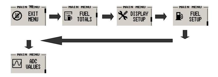
**Note:** ("ADC Values" menu item is only visible when powering up the unit and pressing the rotary control). The text "CALIBRATE" will appear on the intro screen when entering this mode.
