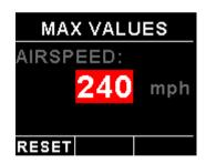
This display can be accessed by rotating the rotary control during the normal display mode. Press the F1/Up button when the max values display is showing to reset the maximum values to the current airspeed.
