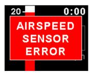
Airspeed sensor error. The instrument could have a faulty airspeed sensor in which case the instrument will then have to be returned to the factory.
