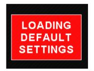
Press and hold the F1/Up button and rotary control during power up to load the preprogrammed factory default settings. The following screen will be displayed:
