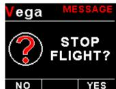
Press the F1/Up button during the normal display mode to manually start/stop a flight. This key is only active if the ASI-4 is setup to select the manual flight option under the "TIMERS" setup menu.
