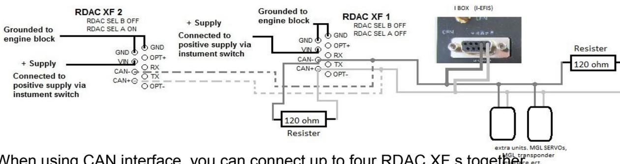
When using CAN interface, you can connect up to four RDAC XF s together.
