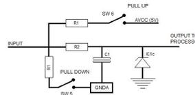
These circuits shows how the various PU switches feeds 5 volt onto the input(sense) line if required. Please check the senders information for type and settings needed. The 2<sup>nd</sup> circuit shows a pull down circuit that has a 100Ω load resistor switched to GND. This intended for use with the Rotax 4-20 mA oil pressure sender. The white wire is connected to the OILP input on the RDAC XF. The OILP PD switch must be in the ON position and the OIL PU switch must be in the OFF position.
