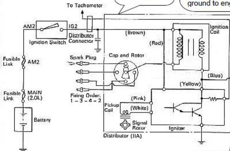
Connect rev counter input on RDAC or instrument to this line. Ensure you have a connection from RDAC ground or instrument ground to engine block.
