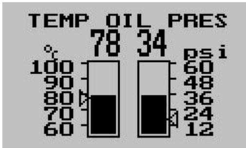
Combined oil temperature and oil pressure display. Most oil sump or dry sump lubricated engines require monitoring of both oil temperature and oil pressure making this option very valuable.
