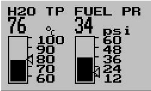
Combined coolant temperature and fuel pressure display. A suitable choice for many water cooled engines.
