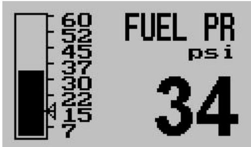
Fuel pressure. The pressure of your fuel supply as measured after the fuel pump and pressure regulator (if any).
