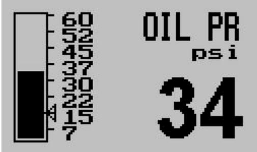
Oil pressure. The pressure of your oil supply as measured after the oil pump / pressure regulator.
