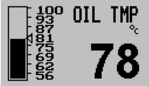
Oil temperature. Usually the temperature of the oil in your sump (crankcase).
