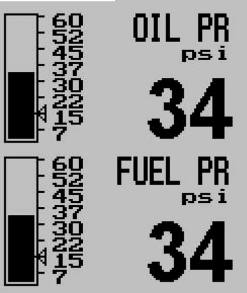
Oil pressure. The pressure of your oil supply as measured after the oil pump / pressure regulator.
