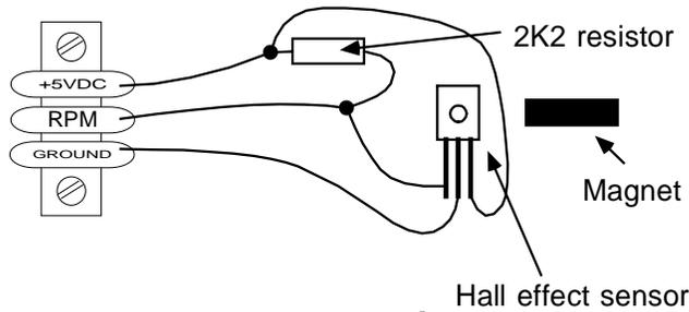
**Typical hall effect sensor installation detects the passing of a magnet suitably fixed to prop flanges or shafts.**
