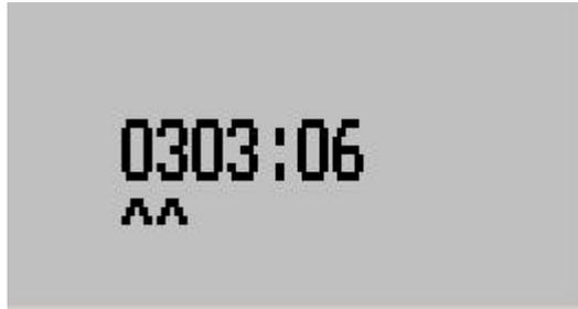
Use the plus and minus buttons to change the indicated part of the hobbs reading. Use the Select button to change from hour hundreds to hours to minutes. End the edit by pressing the Menu button.
