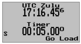
Timer halted, loaded to 5.00 minutes. Press "+" to start the timer.
