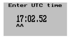
This function is used to set the internal real time clock. The time to be entered must be UTC in order for the system to operate correctly. Do not enter local time (unless it is the same as UTC). UTC is the same as Greenwich Mean Time (GMT) or Zulu time.
