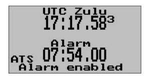
Use the enter key to select the above alarm display. You can use the "+" and "-" buttons to enable or disable the alarm. The alarm time is entered in the menu.
