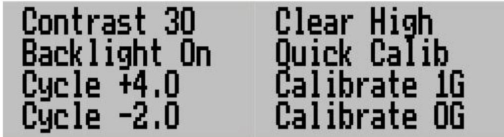
Technical setup functions “Calibrate 1G” and “Calibrate 0G” are accessible if you start up the instrument while pressing both “+” and “-” buttons at the same time
