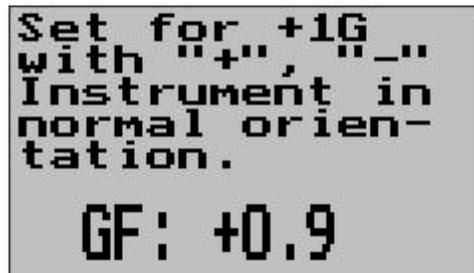
Press "+" to increase the force reading and "-" to decrease the reading. Approximately four key presses are required for 0.1G.
