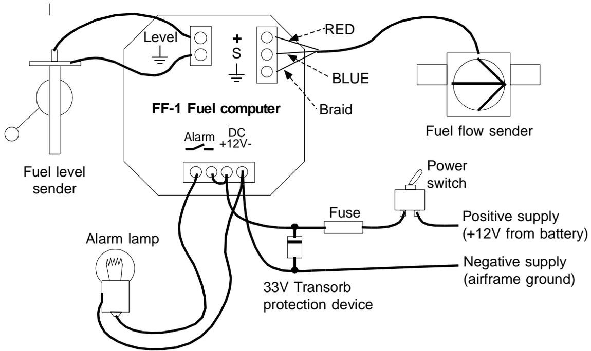
If required the FF-1 can interface to a standard automotive fuel level sender as indicated. Most of these senders are resistive types.
