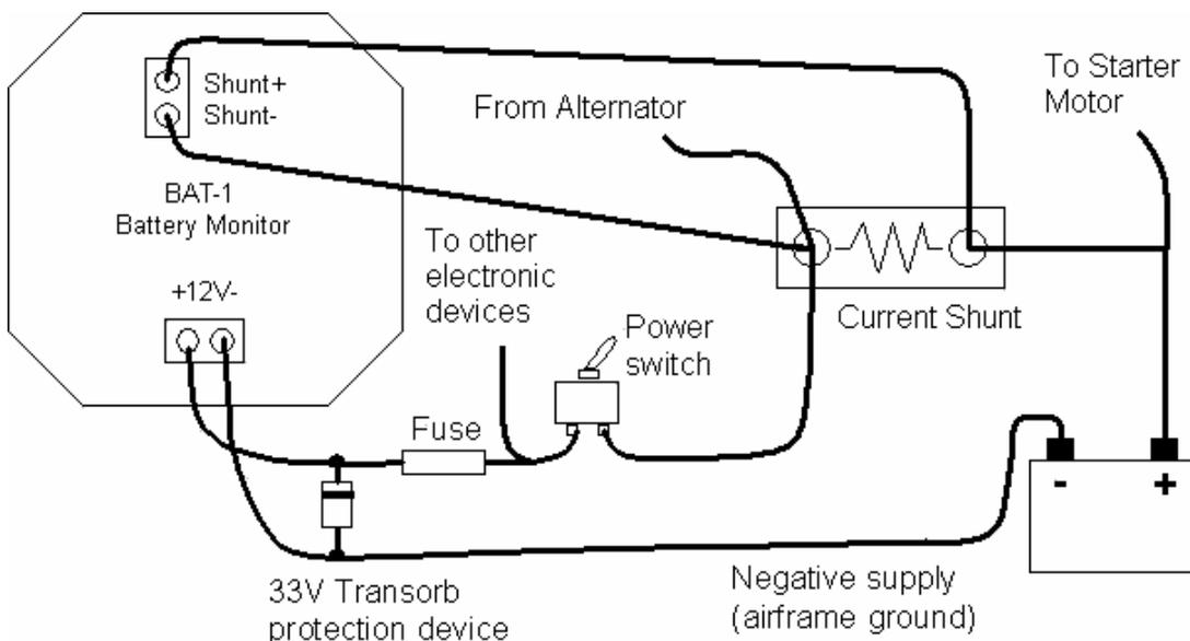
Connect the supply terminals to your aircrafts power supply (you need a dropping resistor or pre-regulator for 24/28V systems). Install suitable power supply protection if you have a supply that can contain large voltage transients such as can be created by starter motors and solenoids.
