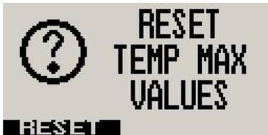
This display can be accessed by pressing the F2 key during the normal display mode. Pressing the F1 key will reset the temporary/current flight maximum values to the current G-force value. Pressing any other key will cause the GF-2 to return to the normal display mode.
