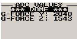
This menu displays the ADC values that have been read from the 2-axis G-force sensor
