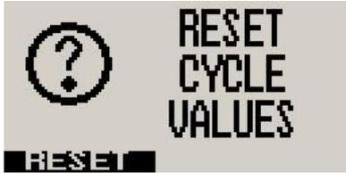
**Note:** The cycle counter values are stored in non-volatile memory and are recalled on power-up.
