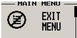
Pressing the rotary control on this menu item will cause the GF-2 to exit the menu system. All changes made during navigation of the menu system will be saved in non-volatile memory on exiting the menu system. If you remove power before exiting the menu the instrument will not save any changes.
