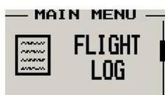
The ASI-1 uses the following algorithm to determine if a flight is in progress (Detect Mode): If airspeed is greater than the preset flight take off airspeed for a duration of 60 seconds or more, a flight is started with a logbook entry. The flight ends if airspeed falls below the preset flight take-off airspeed for 30 seconds. During a flight the logbook cannot be viewed.
