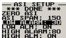
Enter the low airspeed set-point for when the alarm must activate. Any speed below this value will activate the alarm.
