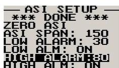
Enter the high airspeed set-point for when the alarm must activate. Any speed above this value will activate the alarm.
