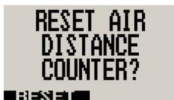
**Note:** The air distance trip counter measures distance flown through the air. This is not the same as distance flown over the ground unless you are flying at sea level at zero wind speed. The air distance shown is subject to under reading at altitude due to decreased air density.
