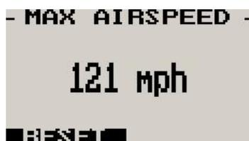
**Note:** The maximum airspeed is stored in non-volatile memory and is recalled on power-up.
