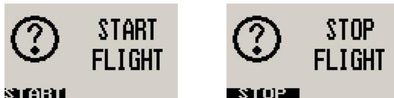
Press the F1 key during the normal display mode to manually start/stop a flight. This key is only active if the ASI-1 is setup to select the manual flight option under the “Flight Log” setup menu.
