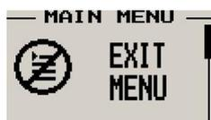
Pressing the rotary control on this menu item will cause the ASI-1 to exit the menu system. All changes made during navigation of the menu system will be saved in non-volatile memory on exiting the menu system. If you remove power before exiting the menu the instrument will not save any changes.
