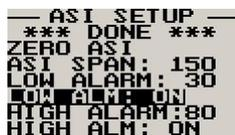
Select whether you want the low air speed alarm to be turned on or off. The low airspeed alarm is only activated once a flight has started.
