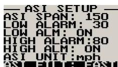
This function can be used to select the signal filter time constant. Selections are "fast" or "slow". This selection influences the rate at which your ASI can change its reading. If you have an installation that suffers from strong turbulence at the pitot tube, select "slow". If you have a very clean airflow in front of the pilot tube you can select "fast" which will give you a faster response to airspeed changes.
