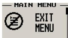
Pressing the rotary control on this menu item will cause the ALT-1 to exit the menu system. All changes made during navigation of the menu system will be saved in non-volatile memory on exiting the menu system. If you remove power before exiting the menu the instrument will not save any changes.
