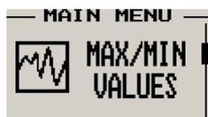
To avoid false recordings, the maximum values function is only activated 10 seconds after the instrument has powered up.
