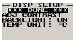
Move the highlight over this menu option and press the rotary button to return to the main menu.
