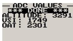
This menu displays the ADC values that have been read from the pressure sensors.
