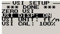
Select if you want to show the built in VSI (vertical speed indicator). The built in VSI will be shown above the altitude readout.
