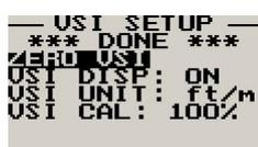
This function is used to set your VSI to read exactly 0ft/min. This is similar to setting the needle on a mechanical VSI to point to zero by turning the adjustment knob on such a VSI. The electronic VSI generally has much less drift compared to a mechanical VSI and this function will only be used very occasionally. Ensure that you perform this function when no pressure changes due to wind or other reasons are occurring.
