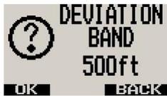
Adjust the deviation band above and below your reference altitude that is still acceptable to fly in. Any altitude outside this band will activate the alarm. Press the F1 key to accept, press the F2 button to return to the main display.
