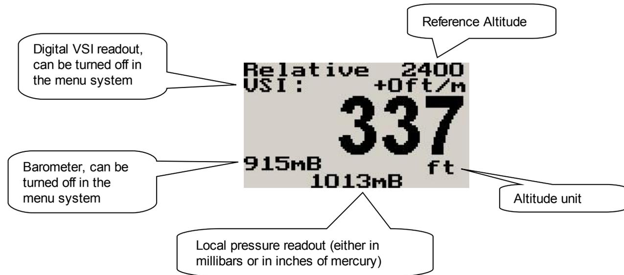
Use the rotary control to adjust the local pressure setting. Pressing the F1/up key will allow the pilot to enter a reference altitude.
