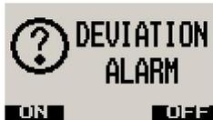
Select whether you want the altitude deviation feature enabled or not. Press the F1 key to enable the altitude deviation feature, press the F2 key to disable the altitude deviation feature.
