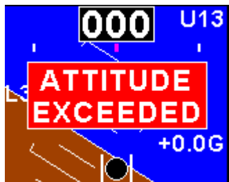
Message displayed when the maximum bank, pitch or yaw rates have been exceeded
