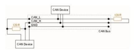
The connection uses two wires which are twisted around each other. This forms a "balanced transmission line". It helps to reduce emissions and also makes the link more robust against external interferences.
