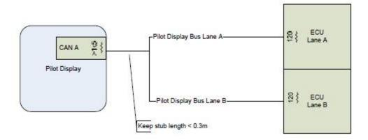
As shown on this diagram, connect the CAN bus ECU lanes A and B together and then connect to the RDAC CAN "CAN ECU" inputs.
