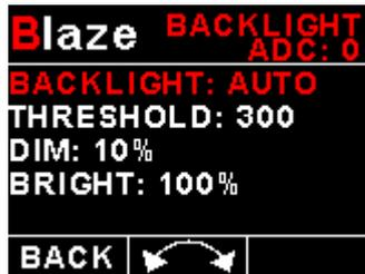
Allow 3 seconds for the display to adjust to the ambient lighting conditions when using the automatic backlight mode. The display will set the backlight to the dim setting if the ambient light is less than the threshold setting, alternatively the display will set the backlight to the bright setting if the ambient light is greater than the threshold setting. The ambient light received is shown as the ADC value in the top header. Use this value to set the threshold value.
