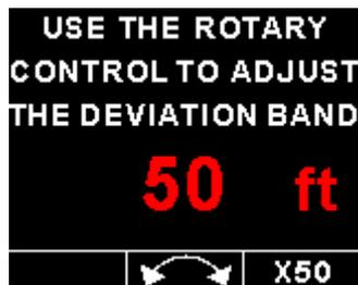
Use the rotary control to adjust the altitude deviation band. Press the F2/Down key to change the increment / decrement unit to 50 or 100. Press the rotary control to exit and save.
