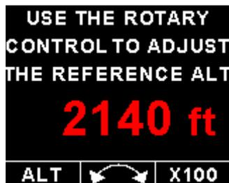
Press the F2/Down button during the Relative Altitude display to access the altitude reference screen. Press the F1/UP key to set the reference altitude to the current altitude or use the rotary control to adjust the reference altitude. Press the F2/Down key to change the increment / decrement unit to 10 or 100. Press the rotary control to exit and save.
