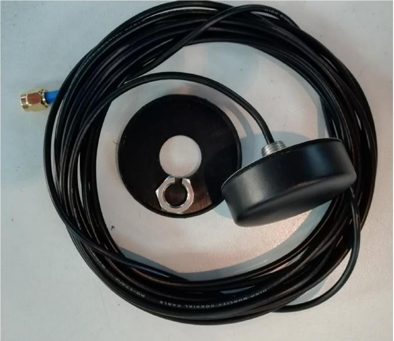
The GPS antenna is an active “patch” type antenna mounted inside a circular “hockey puck” protective housing. This antenna must be installed such that the puck flat surface faces up (so the cable connection faces down towards the Earth).
