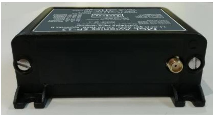
The SP-12 provides a SMA type antenna port at the rear of the SP-12 housing. The SP-12 is designed to support only active GPS antennas that have a supply voltage range from 3.0 to 3.3V DC. Most active GPS antennas on the market today would be compatible with this requirement. The SP-12 is not intended to be used with passive GPS antennas.
