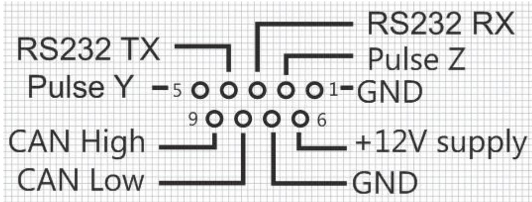
Pinout of the connector of the SP-12. If you are wiring up a male counterpart, this layout is applicable to the view on the solder or cable side of the connector.
